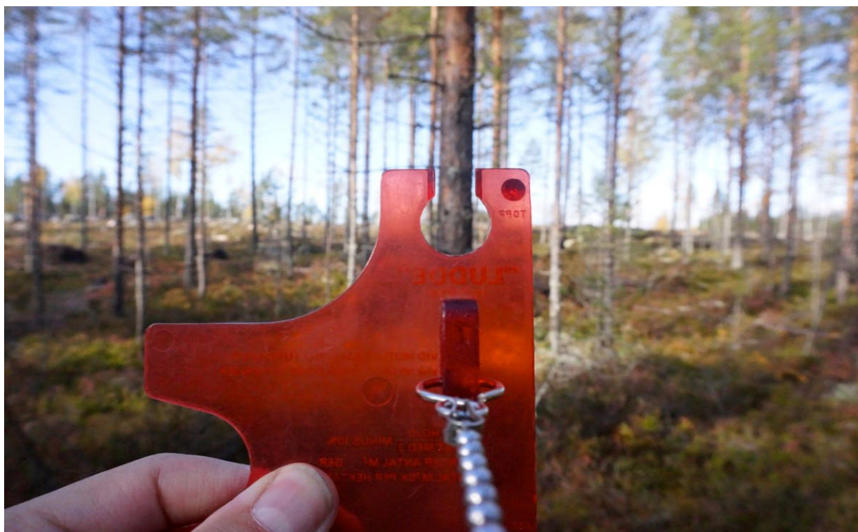
Figure 2.2.3d. Relascope (Ludde) method to score tree stems. Stems that fall inside the relascope gap are not scored (such as the pine tree shown); those that are equal to or larger than the gap are scored.
